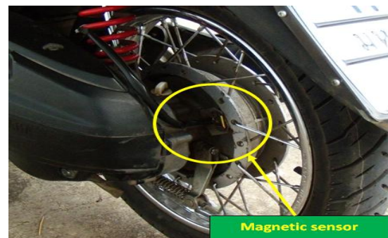
Fig. 4 Magnetic Sensor on Rear Wheel of Motorcycle
