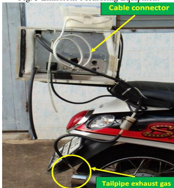
Fig. 6 Emission Measuring Unit Installed on Rear Side of Motorcycle
