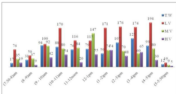
**Fig. 11** Traffic flow by mode at station 3
