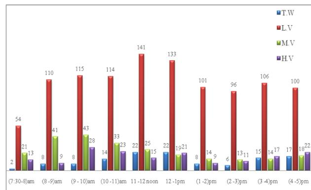
**Fig. 3** Traffic flow by mode at station 1
