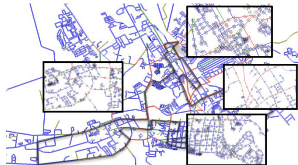
Figure 7 Estimated Vehicular Velocity along the Roads in Iloilo City from JICA STRADA Incremental Assignment Results
