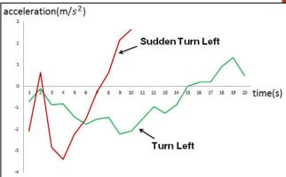
Figure 6 Example of raw data collected from accelerometer sensors illustrating turning events
