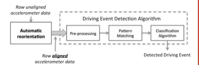
Figure 7: The use of Automatic Smartphone Reorientation in Driving Event Detection
