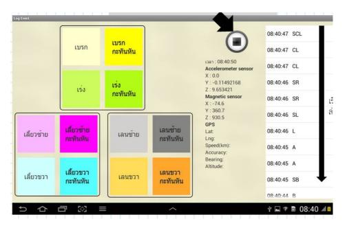
Figure 17 Driving data collector application
